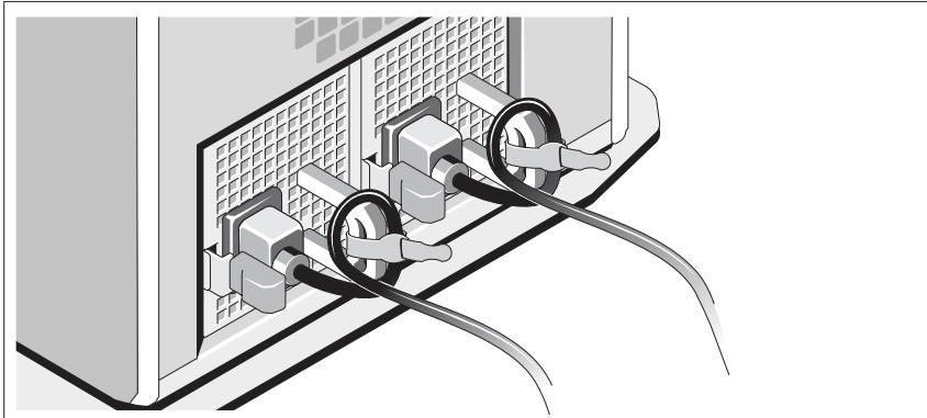
Bend the system power cable into a loop as shown in the illustration and secure the cable to the bracket using the provided strap.
